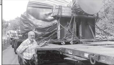
Phillip Schmidt, President and Chief Engineer of Schmidt Equipment, Inc. of Geneva, stands by supports the company designed and built for use in transporting a 140-ton turbine from Louisiana to a company on the east side of Cleveland.
